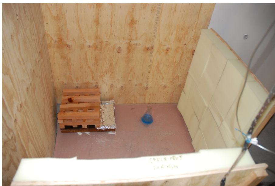
Figure 5 View of the ignition point and surrounding props in Test 1
