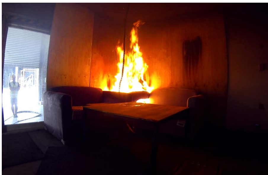
Figure 61 View of the test fire before sprinkler activation
