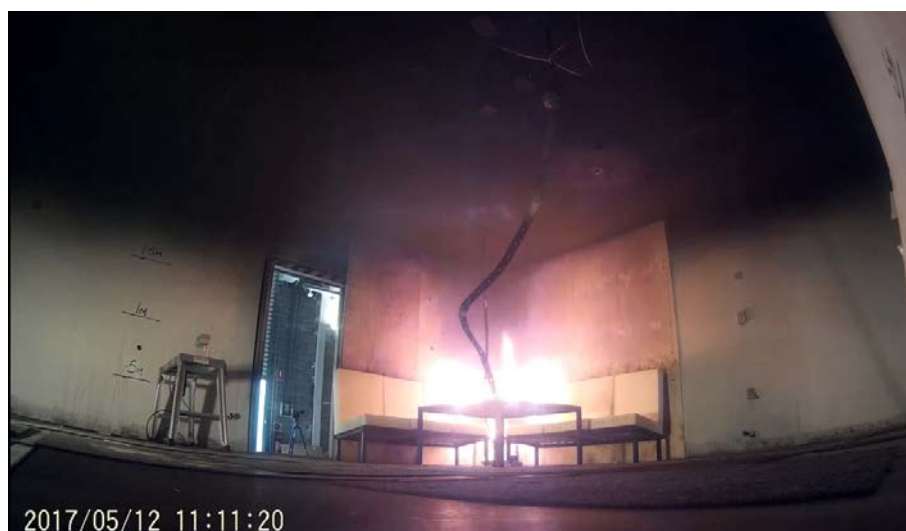
Figure 74 View of the test fire before sprinkler activation
