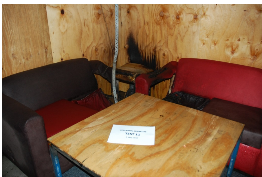
Figure 69 View of the test furnishings at the end of Test 11
