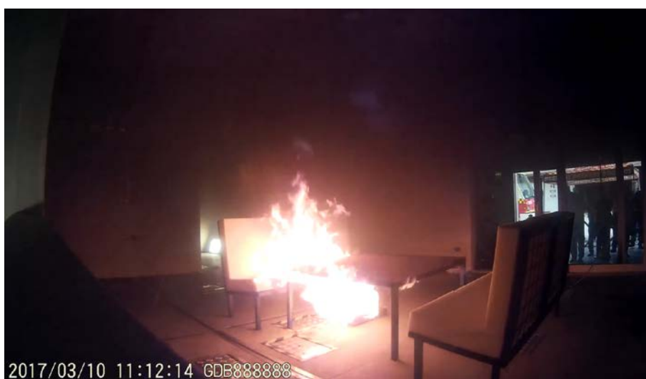
Figure 19 View of the test fire before sprinkler activation
