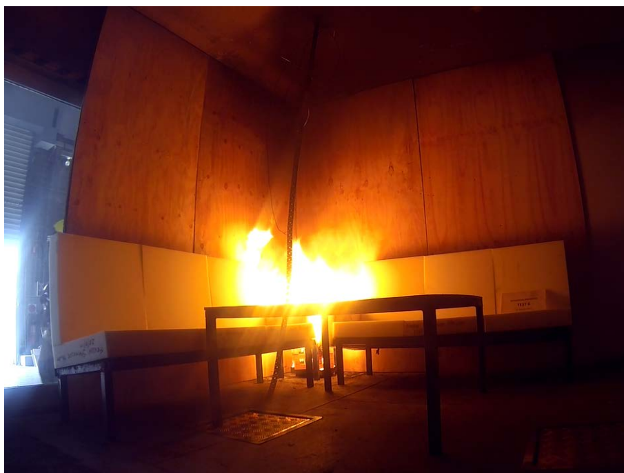
Figure 37 View of the test fire before sprinkler activation during Test 6
