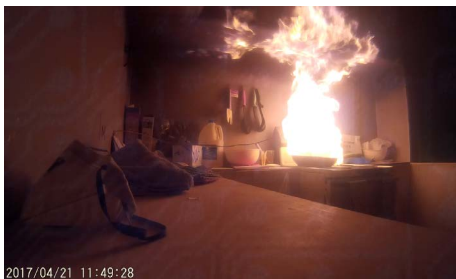
Figure 55 View of the test fire before sprinkler activation
