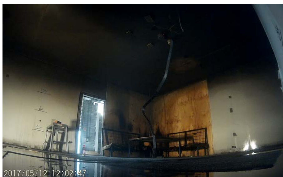
Figure 75 View of the test furnishings at the end of Test 12
