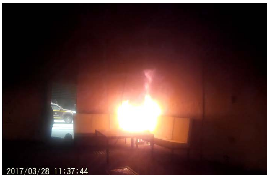
Figure 31 Views of the test fire before sprinkler activation
