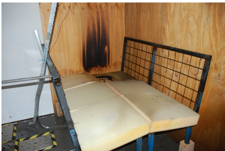
Figure 50 View of the test furnishings at the end of Test 8
