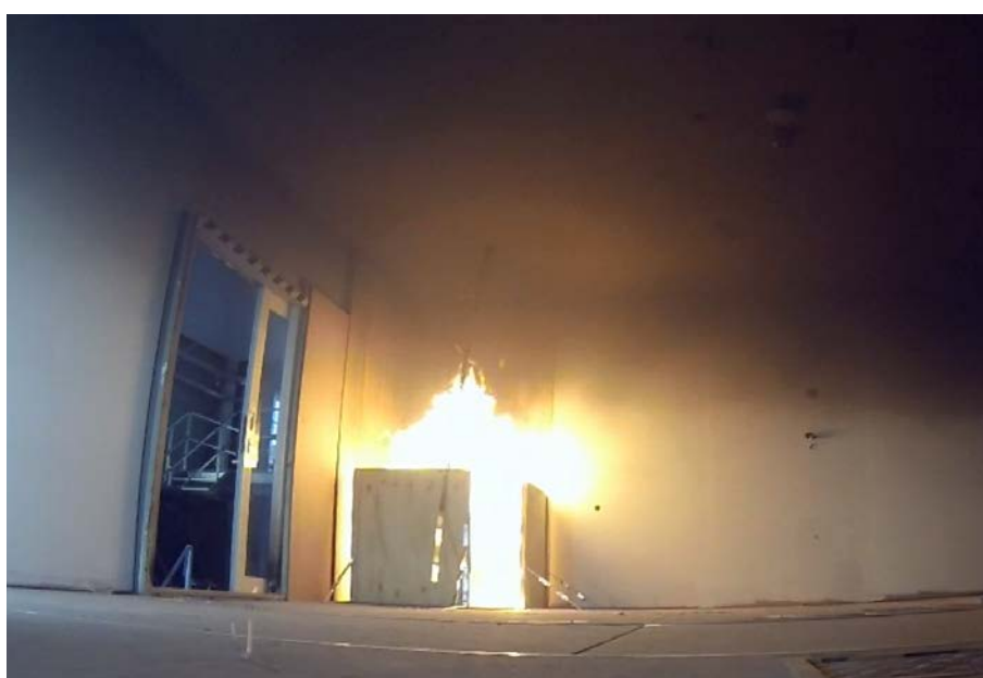
Figure 7 View of the test fire before sprinkler activation
