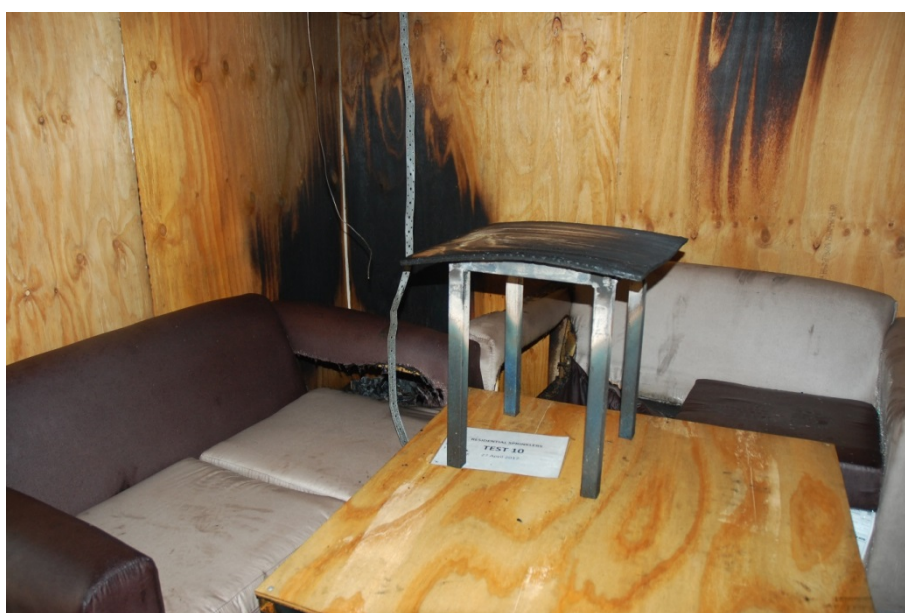
Figure 62 View of the test furnishings at the end of Test 10
