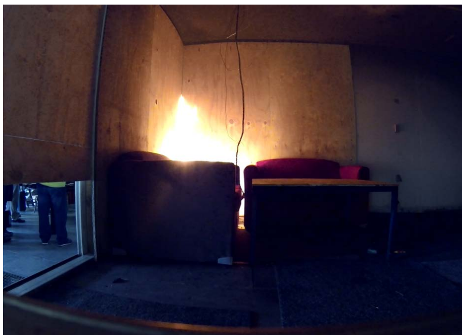
Figure 68 View of the test fire before sprinkler activation
