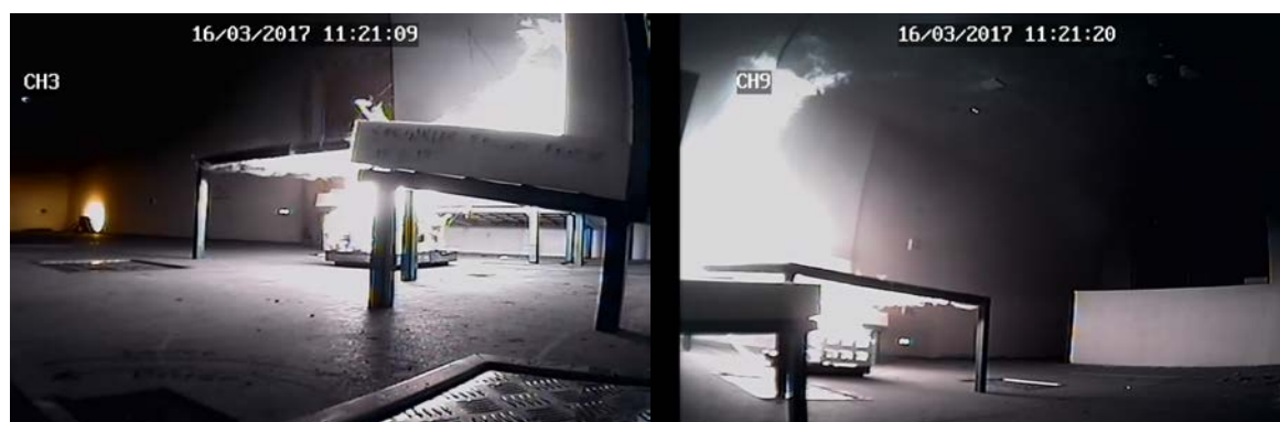
Figure 25 Views of the test fire before sprinkler activation
