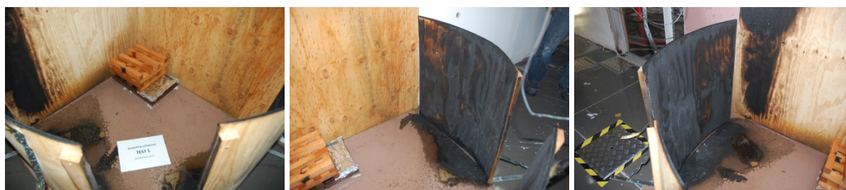
Figure 8 Views of the timber crib and foam panels at the end of Test 1
